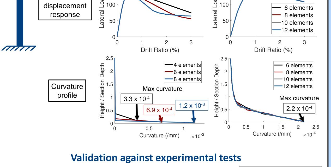
The nonlocal model was validated against a suite of 24 cyclic experimental tests on RC columns. Representative results are displayed.
