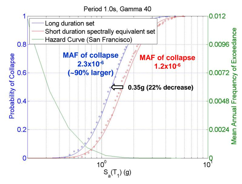
Even a small decrease in median collapse capacity could result in a large increase in the computed MAF of collapse
