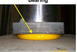
Placed in series with posttensioning bar to prevent premature yielding and loss of post-tensioning.
