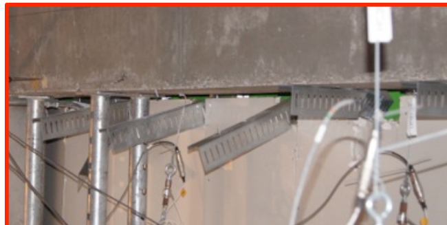
Balloon framing clip detachment
