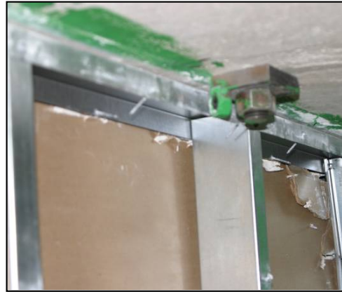
Crushing and shearing of gypsum around screws in connection to top track
