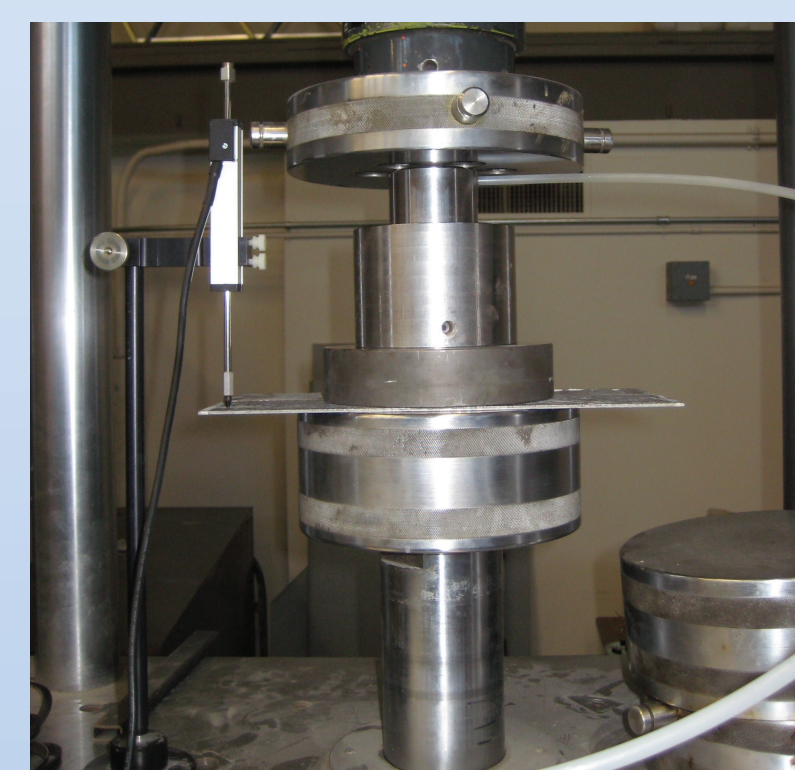
Figure 6 Lower arm of MTS compression frame moves upward to compress soil sample.
