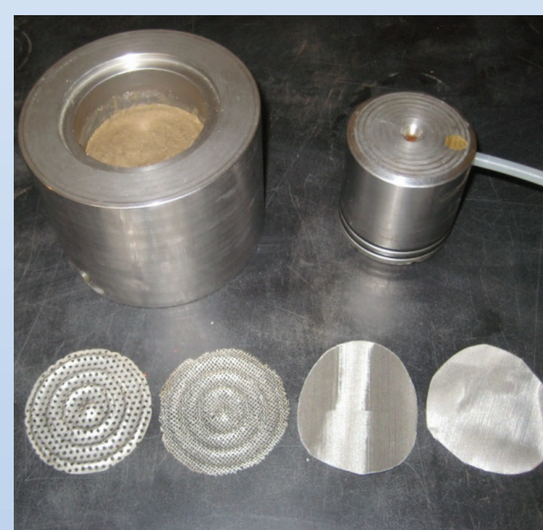
Figure 5 Soil placed in steel mold with drainage screens in preparation for compression.
