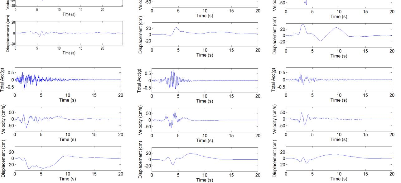
GM realizations for fixed earthquake source and site characteristics: F = 1,  $M_w = 6.2$ , R = 10km,  $V_{s30} = 600$  m/s,  $\theta = 1.0^o$ , s = 27 km; one recorded (top left) and three simulated pulselike near-fault GMs
