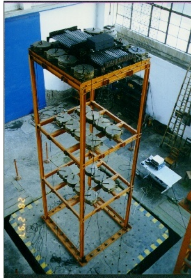
3-story steel frame model in testing
