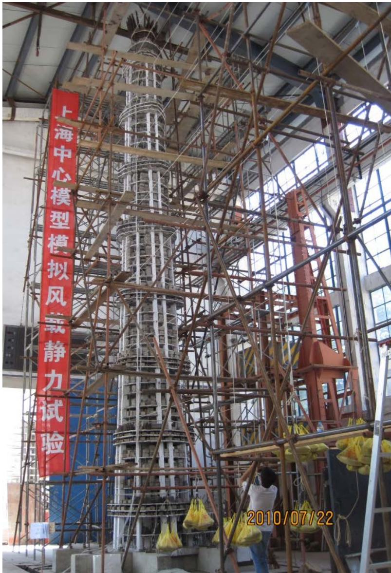
Model test on Wind Loading at Tongji (1/50 scale, 2010.7.20)
