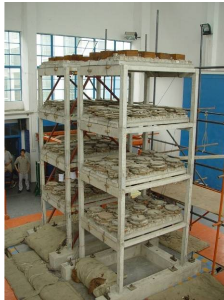
Shaking table model test of R.C. frames with or without dampers
