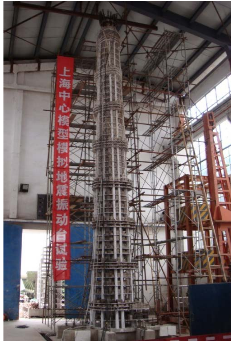
Model test on shaking table at Tongji (1/50 scale, 2010.7.30)
