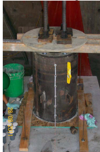
Column + Footing Assembly
