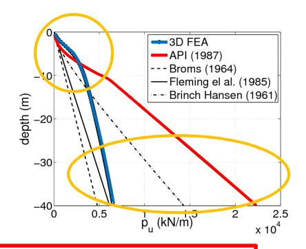
Use of one of the smaller distributions is recommended for p-y analyses of lateral spreading or other load cases in which deep soil-pile interaction is anticipated.
