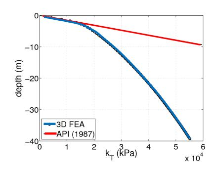
A parabolic distribution of initial stiffness, as used by Brandenberg et al. (2007) and Lam and Cheang (1995), or a similar bilinear distribution to that above is recommended for a static BNWF analysis of lateral spreading.
