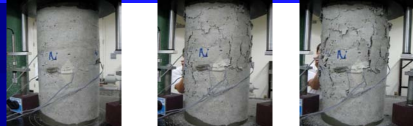
SC-HyFRC: delay in damage initiation and damage progression
