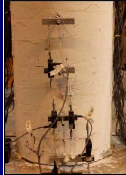
Self-compacted HyFRC column \rho_v=0.37\%
