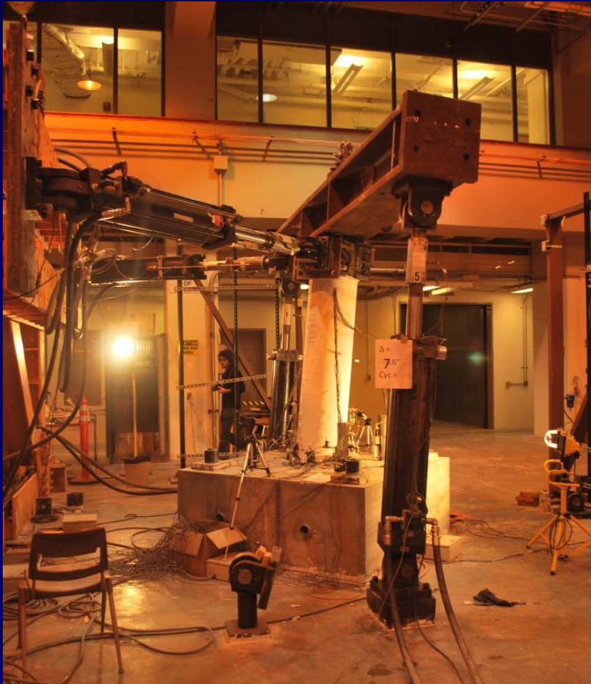
Self-compacted HyFRC column during 11% drift
