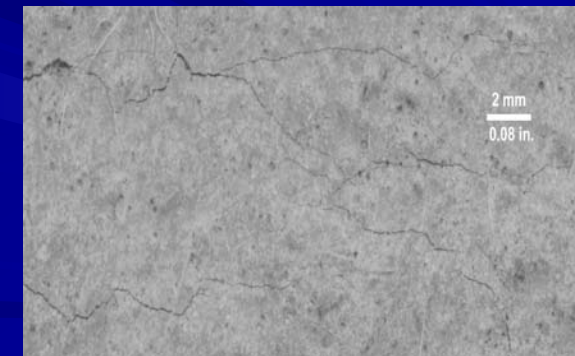
Only Microcracks formed in HyFRC after 5 cycles despite double the load level
