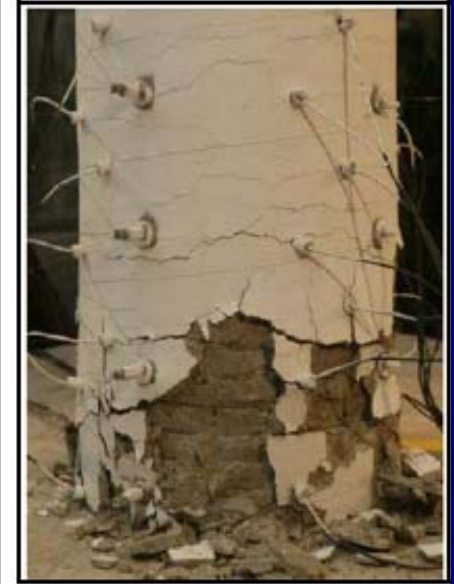
Conv. reinforced concrete column \rho_v=0.70\%
