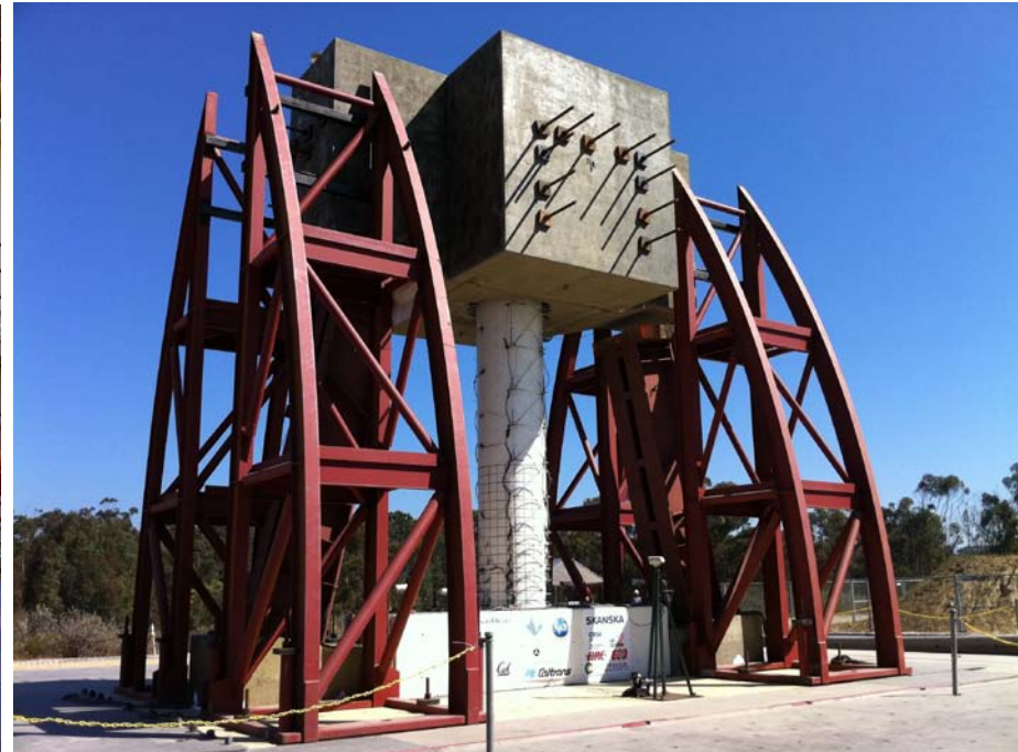
Full-scale 1D tests of circular column - Jose Restrepo, PI (PEER, Caltrans, UNR, FHWA, NEES@UCSD, NEES & NSF)
