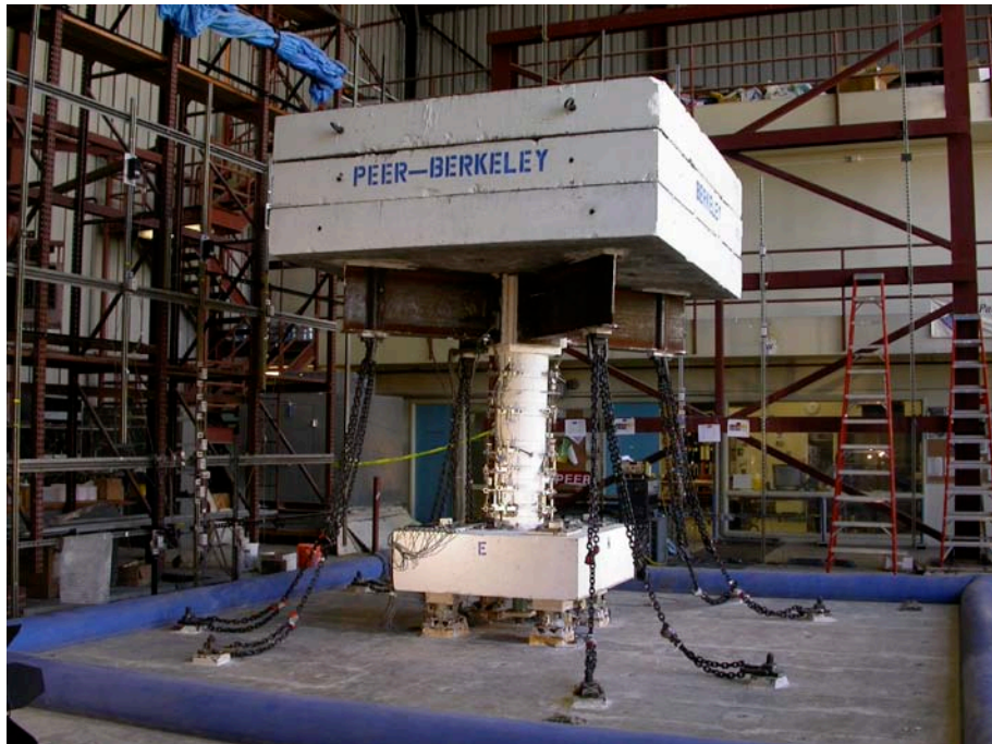
Reduced-scale 3D tests of conventional circular and rectangular columns, self-centering columns, rocking columns (PEER)
