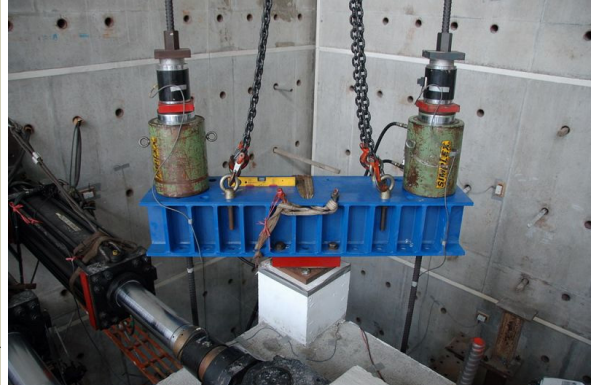
Fig. 10. Photo of vertical loading system
