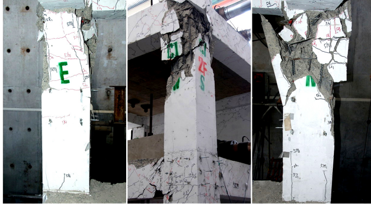
Fig. 24. -3% 2 nd cycle: C1-2F collapse
