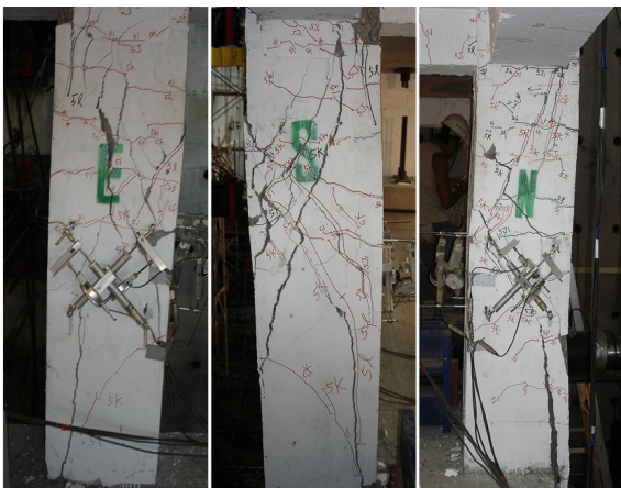
Fig. 22. +3% 1 st cycle: C2-2F shear failure
