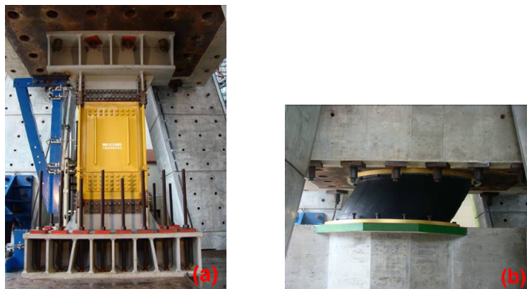
Fig. 5. Test setups for (a) a viscous damping wall and (b) a LRB
