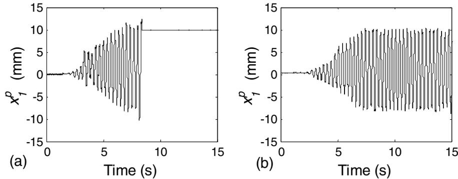
**Fig. 3. Experimental results of a Single-DoF split-mass system, excited by a sinusoidal force with  $A=10 \text{ N}$  and  $f=3 \text{ Hz}$ , by using (a) the Chang's method, (b) the LSRT2 method.**
