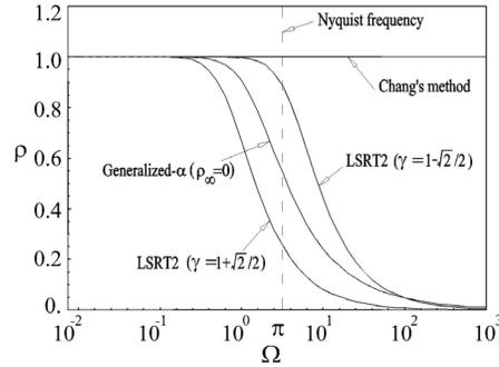
**Fig. 2. Spectral radii  $\rho$  of linearly implicit algorithms with respect to the Generalized- $\alpha$  method vs. the non-dimensional frequency  $\Omega$ .**
