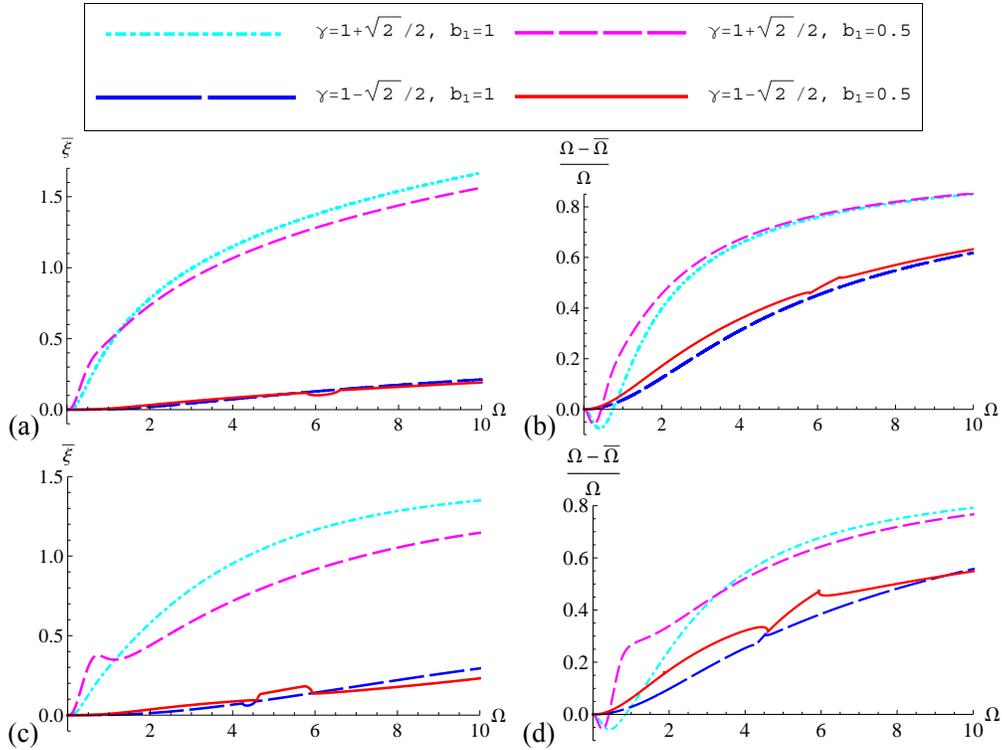
**Fig. 6.** Algorithmic damping ratio  $\bar{\xi}$  and relative frequency error for the staggered procedure: (a), (b)  $ss=1$ ; (c), (d)  $ss=10$ .
