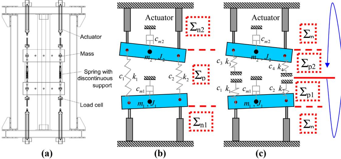
**Fig. 9. Test rig: (a) experimental set-up; (b) and (c) schematic configurations of numerical and physical substructures.**
