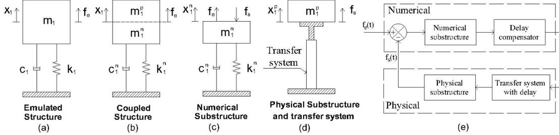
**Fig. 1. (a)-(d) Schematic representation of a SDOF split-mass system; (e) block diagram representation including delay.**
