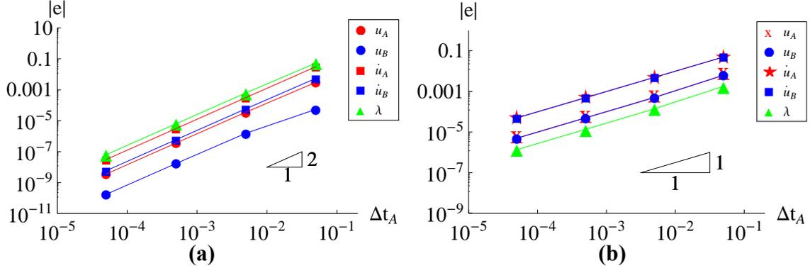
**Fig. 7. Global error for the staggered procedure with  $b_1=0.5$  and  $ss=10$ : (a) the LSRT2 algorithm with  $\gamma = 1 - \sqrt{2}/2$ , (b) the midpoint rule algorithm.**
