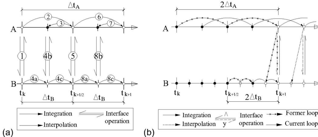
**Fig. 4. The multi-time-step partitioned algorithm with  $ss=2$ : (a) staggered procedure; (b) interfield parallel procedure.**
