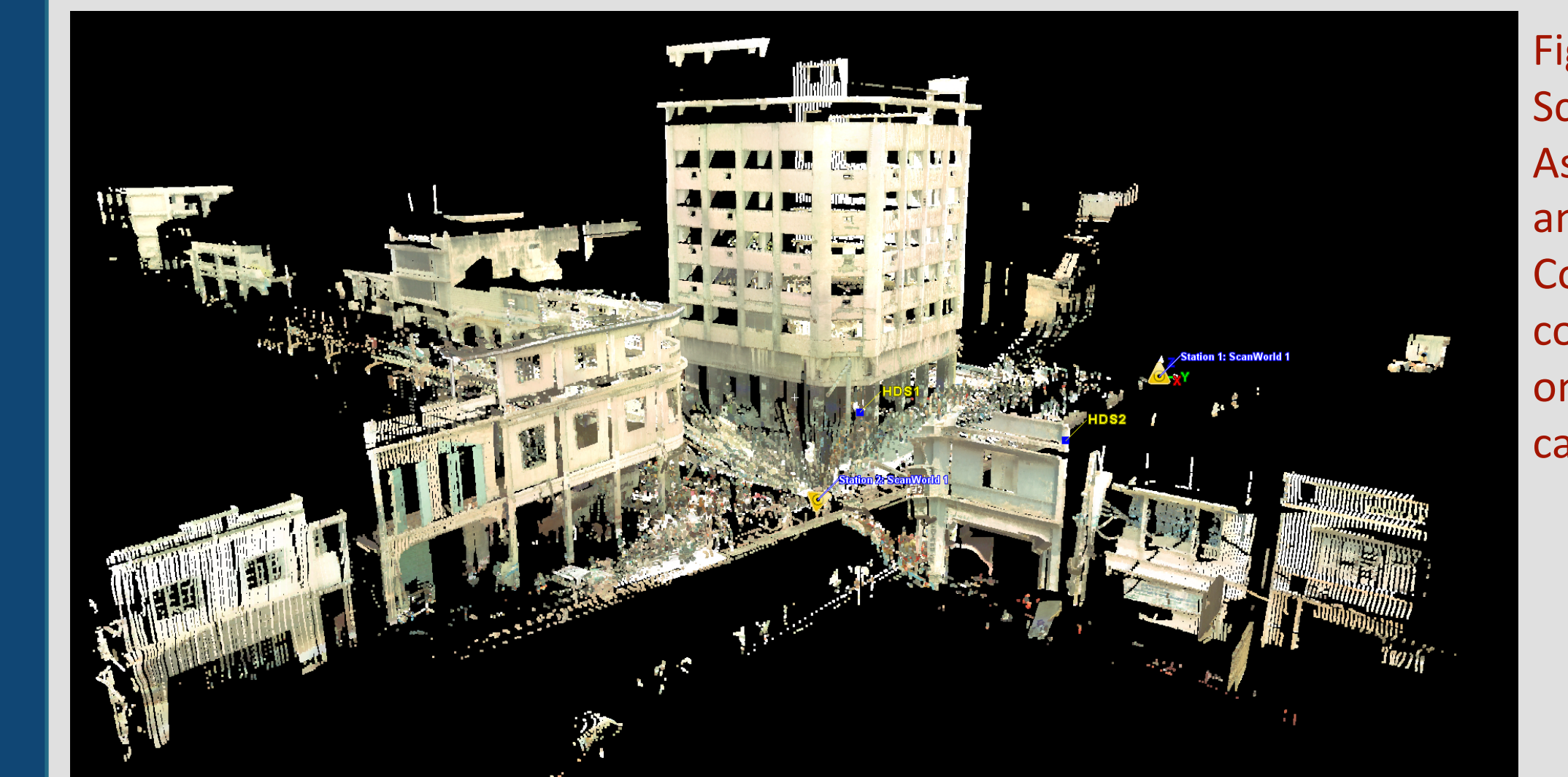
Figure 9: Laser Scan of the Asscotia Hotel and intersection. Colored by the colors from the on board camera.
