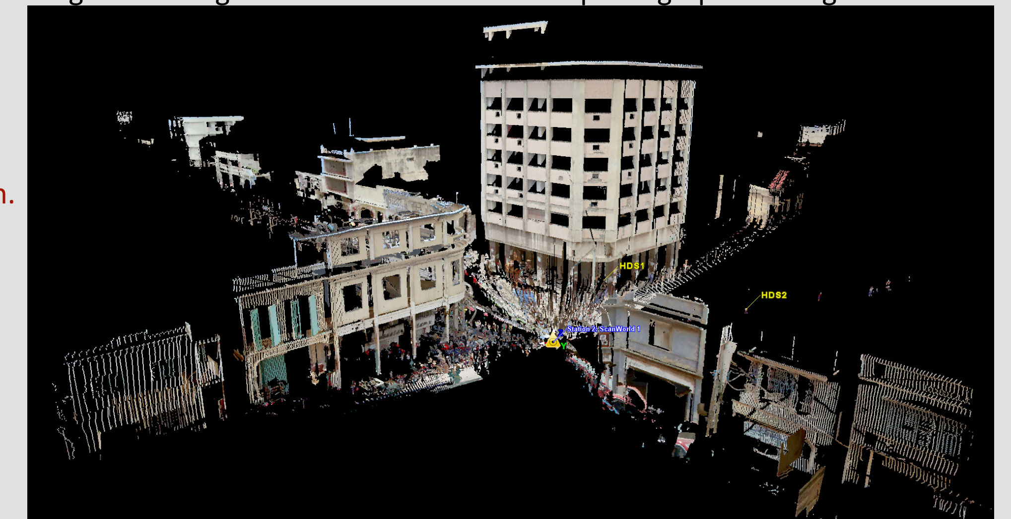
Figure 9: Laser Scan of the Asscotia Hotel and intersection. Colored by the colors from the on board camera.
