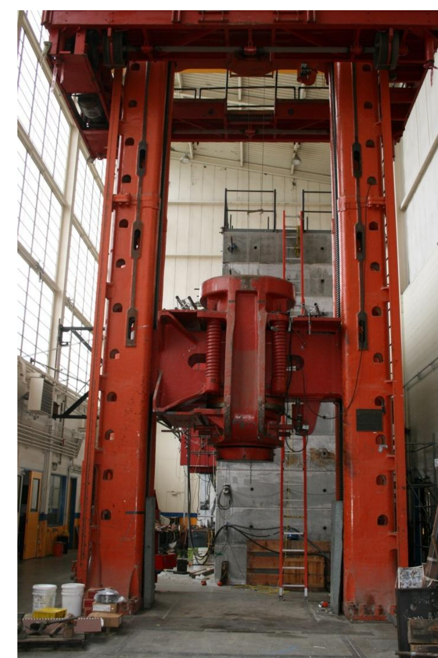
Figure 8: "Big Press" 4,000 kip capacity compression machine
